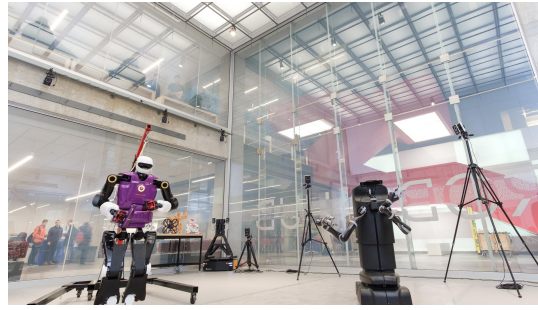
(a) A humanoid, a mobile manipulator, and the ceiling camera system in the Robohub.
